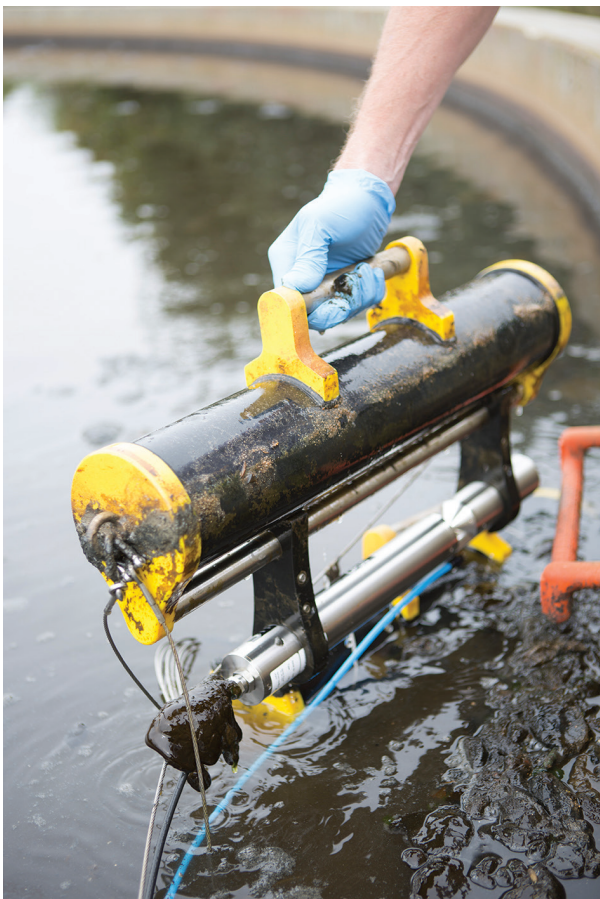
Measurement of nitrates and nitrites in a treatment station, mounting OPUS probe on a float with automatic cleaning by injection of compressed air
