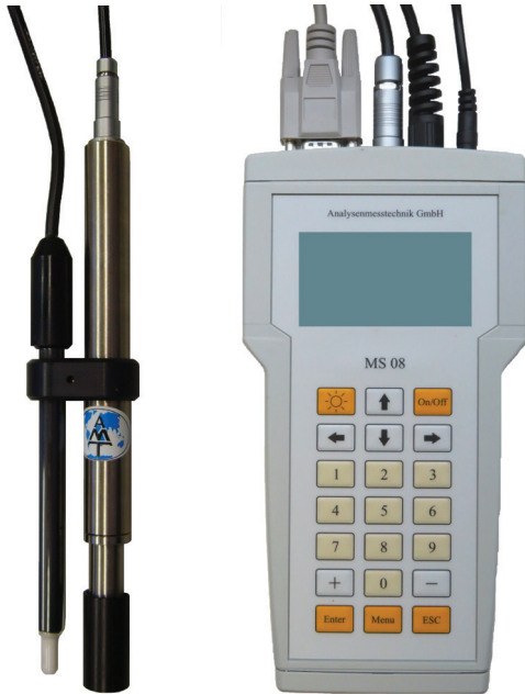
Multi-parameter system Adapt to micro-sensors H 2 S - H 2 - H 2 O 2 - O 2 - O 3
