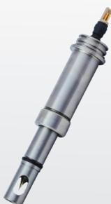
The dissolved H<sub>2</sub>S passes through the gas permeable membrane. It diffuses to the working electrode where an electrochemical oxidation reaction operates. The current generated, proportional to the hydrogen sulphide concentration, is measured by the probe.
